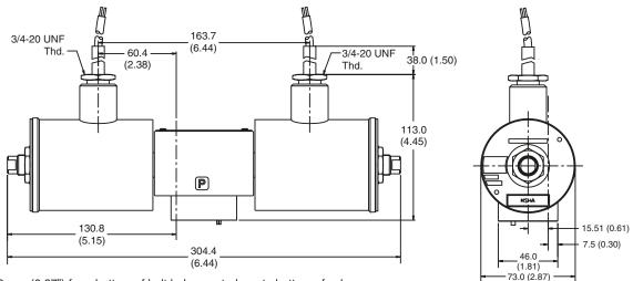
Note: 22.0 mm (0.87") from bottom of bolt hole counterbore to bottom of valve.
