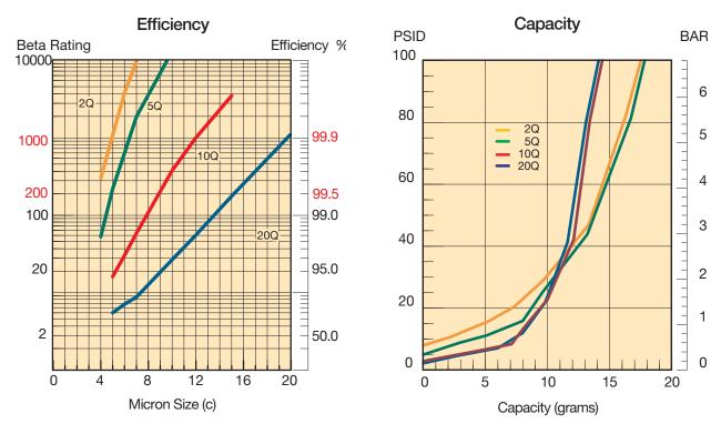
Results typical from Multi-pass tests run per test standard ISO 16889 @ 15 gpm to 100 psid terminal - 10 mg/L BUGL Refer to Appendix on pages 265-266 for relationship to test standard ISO 4572.
