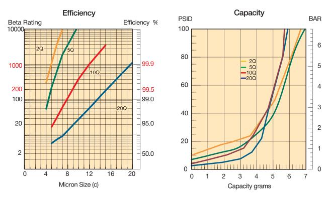
Results typical from Multi-pass tests run per test standard ISO 16889 @ 10 gpm to 100 psid terminal - 10 mg/L BUGL Refer to Appendix on pages 265-266 for relationship to test standard ISO 4572.
