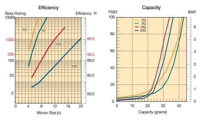
Results typical from Multi-pass tests run per test standard ISO 16889 @ 30 gpm to 100 psid terminal - 10 mg/L BUGL Refer to Appendix on pages 265-266 for relationship to test standard ISO 4572.
