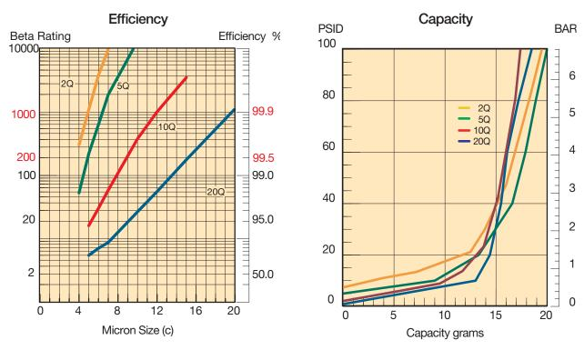
Results typical from Multi-pass tests run per test standard ISO 16889 @ 20 gpm to 100 psid terminal - 10 mg/L BUGL Refer to Appendix on pages 265-266 for relationship to test standard ISO 4572.
